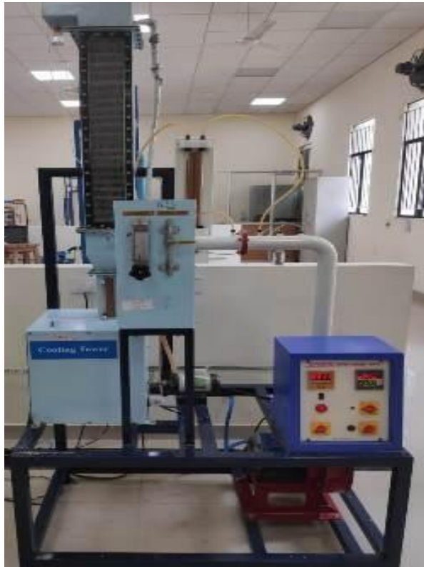
Cooling tower Apparatus
